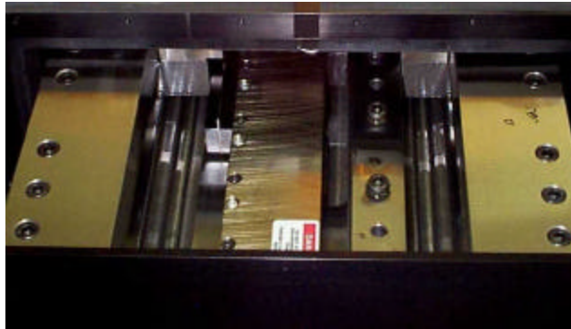
Kinematically Mounted LVDT Tool/wheel Setting System & Linear Motor Driven Hydrostatic Slide
