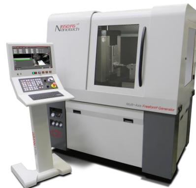
The new HMI is coupled with a 64-bit Delta Tau 1GHz Power PMAC Motion Controller with up to 40,000 block lookahead for advanced trajectory calculations. This highly optimized solution provides improved part program edit speeds via embedded custom software for both quick modifications or full edit functions and
