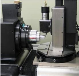
On show will be the most affordable yet technically advanced Nanotech 250UPL, incorporating a high speed air bearing multi-orientation grinding spindle, with a fully CNC controlled Y axis atop its integral indexing table, allowing for WECS on-machine metrology.
